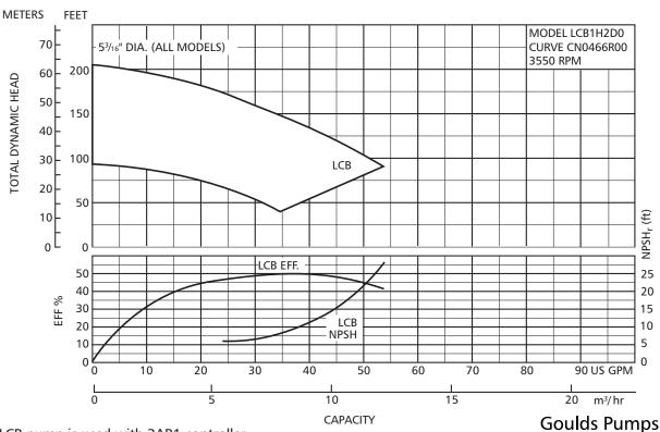
NOTE: LCB pump is used with 3AB1 controller.
